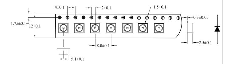
Note: Tolerance unless mentioned is ±0.1mm; Unit = mm
